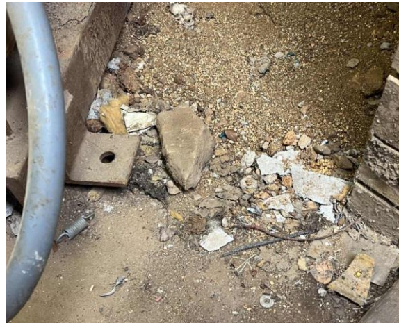
Line ID 134: Internal, Student Lodges, Snowgums Lodge, Basement Plant Room, Adjacent Brick Pillar, Compressed Cement Sheeting Debris - Chrysotile Asbestos Detected
